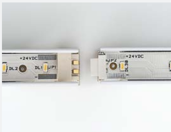
Put plug connector closer to socket connector.
