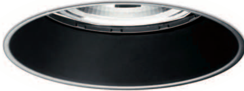
Recessed luminaire Ø 158 mm - Fixed optical component HMG (HALOSPOT111) 100W max - 12V - G53
